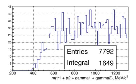
In the hypothesis that the two used tracks are pions I plot the spectrum of invariant mass of two tracks and two photons.
